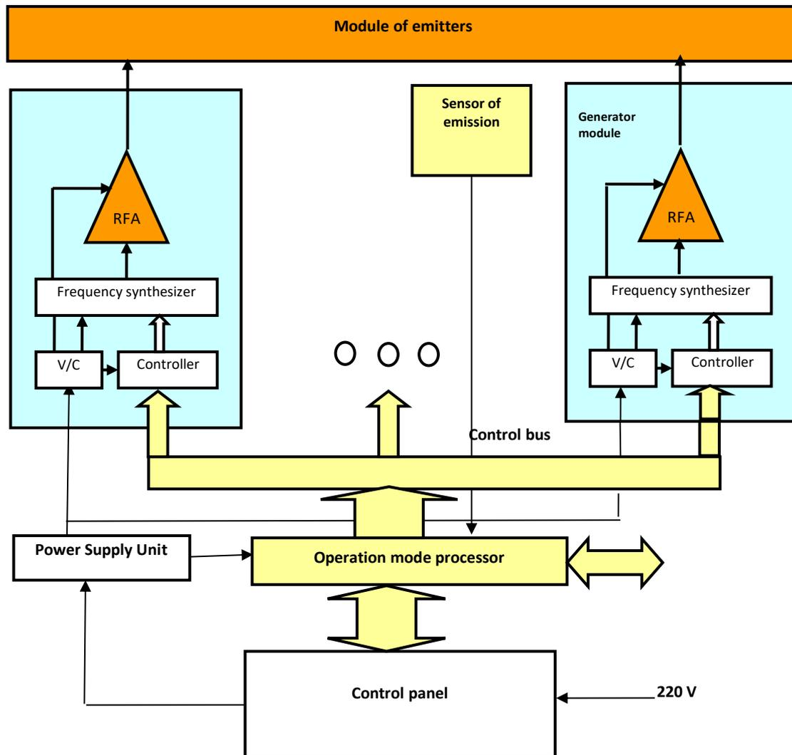
Picture 3.1 Functional Diagram of the device BIOL
