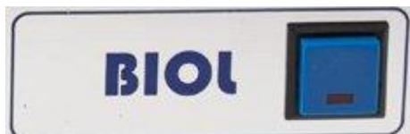
Power indication of the device (the red indicator on the button isn't light when the device is turned off).
