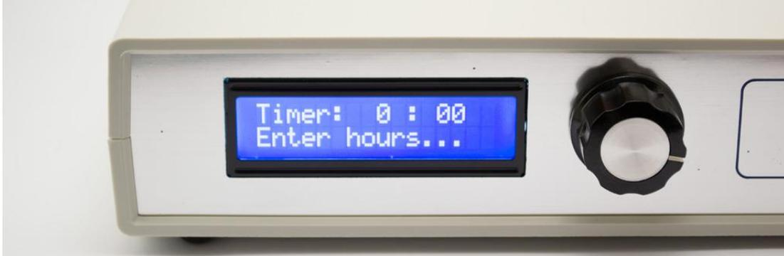
First you need to set the duration of the session in **hours** - «Enter hours...». To start, press the encoder-knob, as a normal button. Then rotate the knob-encoder left or right to select the required number of hours for a session. Set hours by pressing the knob-encoder, as a button.
