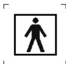
The device is protected by reinforced insulation and has no galvanic connection to the ground
