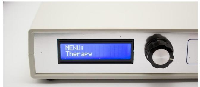
To switch the mode from “Therapy” to “Rehabilitation” or vice versa, roll the knob-encoder left or right. Once the menu you need is displayed, press the encoder-knob, as a normal button. The operating mode of the device is set.
