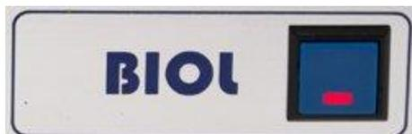
Power indication of the device (the red indicator on the button is light when the device is turned on)..
