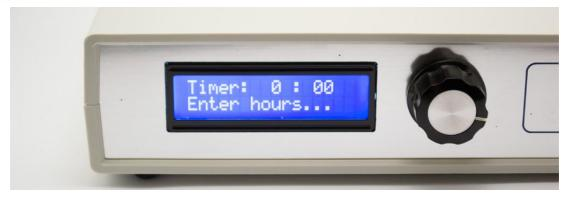
First you need to set the duration of the session in *hours* - «Enter hours...». To start, press the encoder-knob, as a normal button. Then rotate the knob-encoder left or right to select the required number of hours for a session. Set hours by pressing the knob-encoder, as a button.
