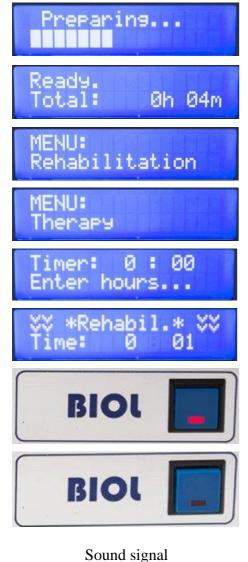
Automatic mode of preparation of the device to work, which includes self-testing and diagnostics of hardware are carried out – "Preparing"
