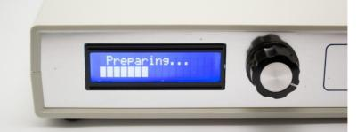
5.4.4 Upon completion of preparing, the device is ready to be used "Ready" and it goes into the standby mode of setting the session parameters. The information about the total operating time of the device is displayed "Total: XXh XXm" (total operating time in hours (h) and minutes (m) since it was manufactured)::
